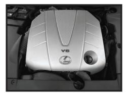
Step 2 Lift up and remove the engine top cover.
