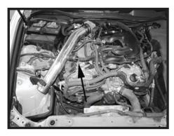
Step 19 Reinstall the crankcase vent hose to the intake tube.
