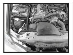
Step 7 Remove the two 10mm bolts that secure the air box to the body. Grasp the air box and pull it out of the vehicle including the fresh air duct.
