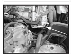
Step 17 Remove the bolt in the right (passenger side) front corner of the valve cover and set it aside as it will be used in a later step.
