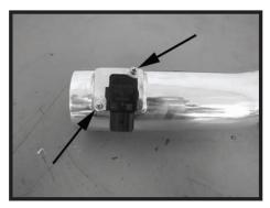
Step 9 Install the MAFS into the Spectre Performance intake tube and secure with the supplied screws.
