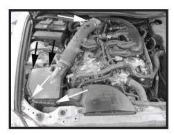
Step 6 Loosen the clamp on the intake tube at the throttle body. Unclip the air box lid and remove the upper air box assembly and filter from the vehicle.
